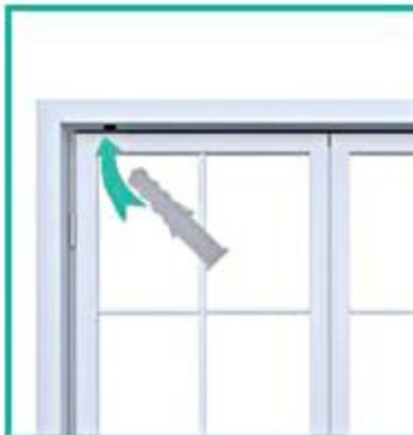
03. Input the plastic screw into the holes
